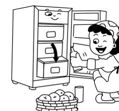
4 Fasten the interior componets with tape.
